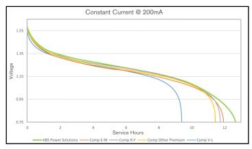
Tested to 60079-11 10.5 direct short circuit until fully discharged with no leakage, suitable for T4 temperature code as a component within intrinsically safe equipment.
